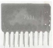
Because of the small and consistent dimensions of the circuitry in the hybrid pack there is the distinct and important benefit of improved high frequency performance. with short lead lengths and low capacitances there is a relative freedom from instability and interference.
